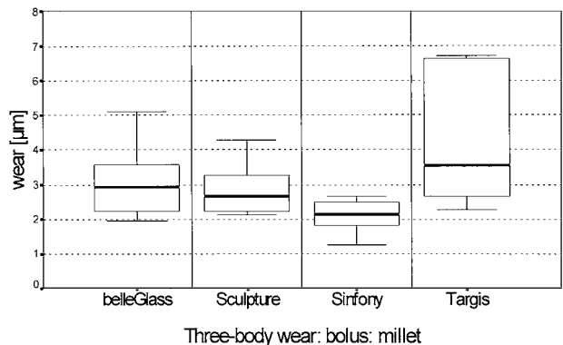
Figure 1 Three-body wear with millet ( \mu\text{m} ) (median, 25%/75% percentiles, min, max).
